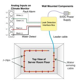
The sensing wire connects to the leader cable which goes to the interface box. Signals from the interface box run to the Geist Climate Monitor.
